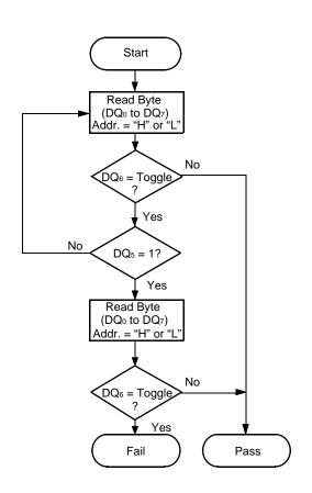
**Note:** DQ $_6$  is rechecked even if DQ $_5$  = "1" because DQ $_6$  may stop toggling at the same time as DQ $_5$  changing to "1".
