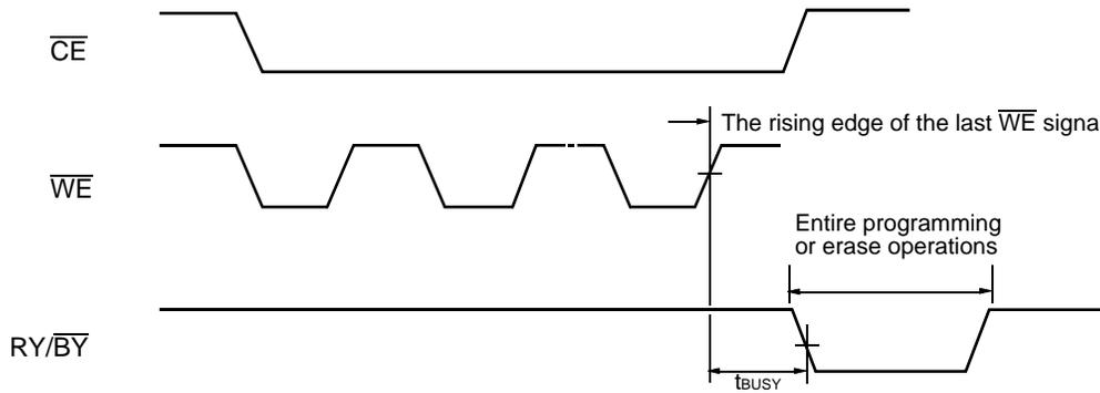
**Figure 11  $RY/\overline{BY}$  Timing Diagram during Program/Erase Operations**
