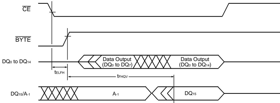
**Figure 13 Timing Diagram for Word Mode Configuration**
