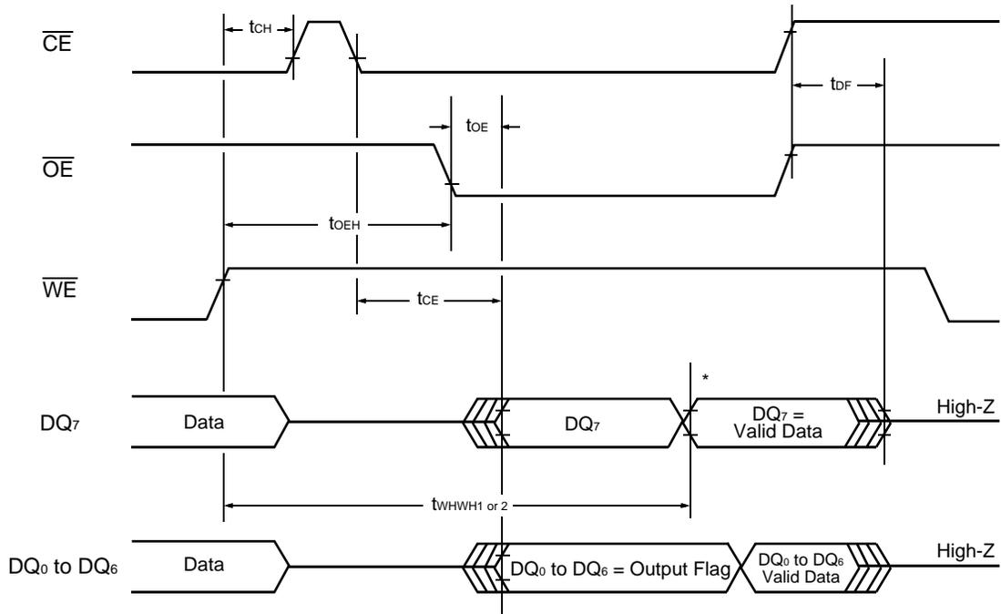
\*DQ7 = Valid Data (The device has completed the Embedded operation).
