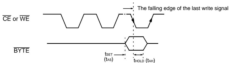
**Figure 15  $\overline{BYTE}$  Timing Diagram for Write Operations**
