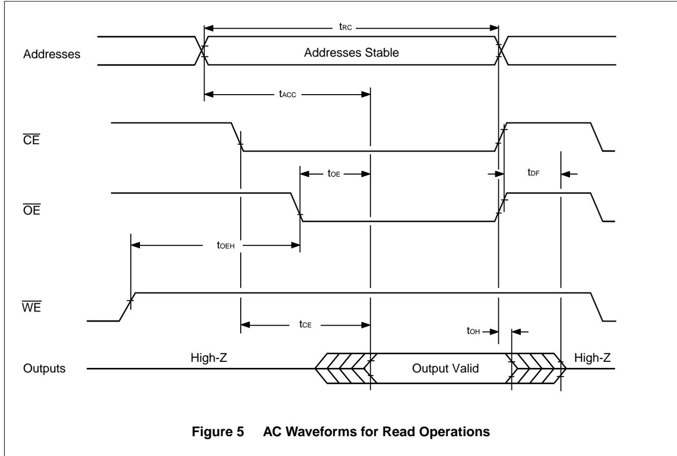
Figure 5 AC Waveforms for Read Operations
