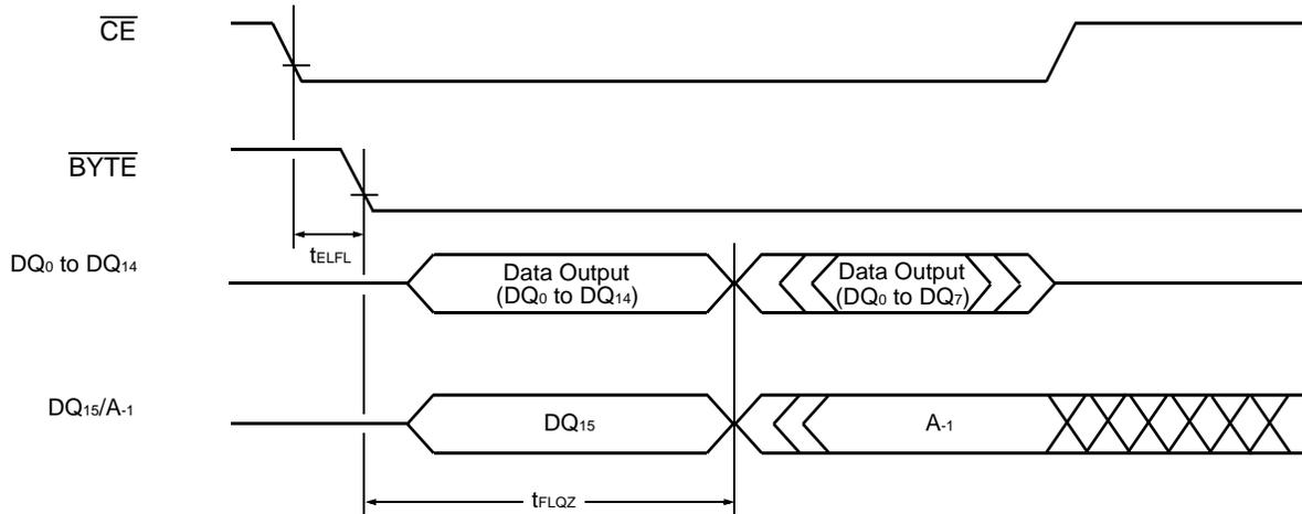
**Figure 14 Timing Diagram for Byte Mode Configuration**
